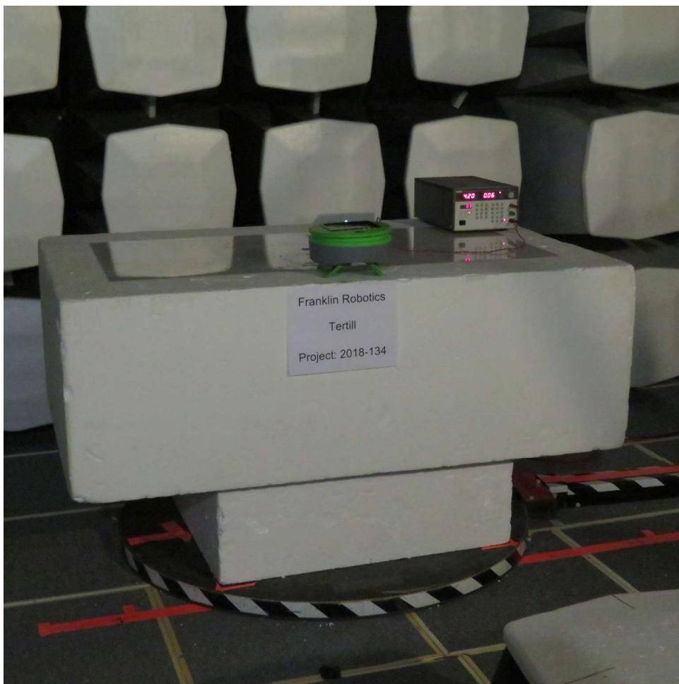
EUT set up in chamber, prescans below 1GHz
