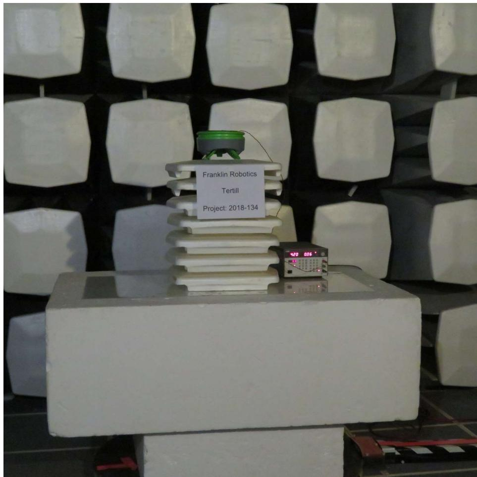
EUT set up in chamber, prescans above 1GHz
