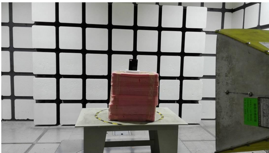
Radiated Emissions View (Above 1 GHz)
