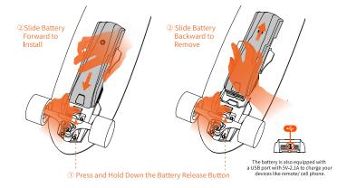
Battery Installation: Align both the ports from the battery and deck. Slide the battery into place, ensuring that it's securely mounted. (Otherwise, it may fall out while riding and cause danger or injury)
