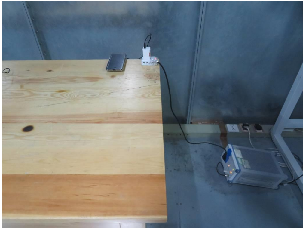
Conducted Emission-AC adapter charge mode
