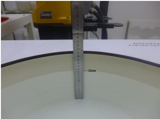
A photograph showing a shallow, curved pool of tissue simulant liquid in a white container. A vertical ruler is positioned next to the container, with the 15cm mark clearly visible. The liquid surface is slightly irregular, reflecting the light. |
