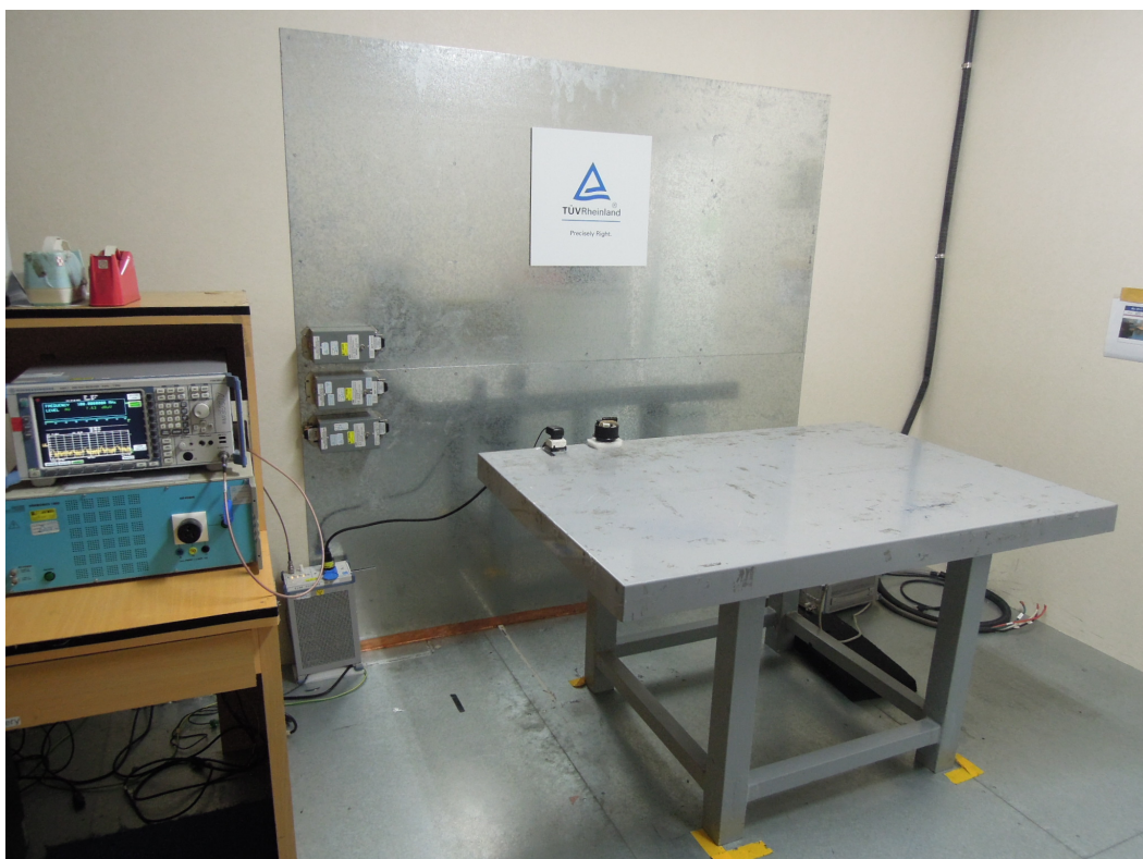
Photograph 5: Set-up for for Mains Conducted testing Front
