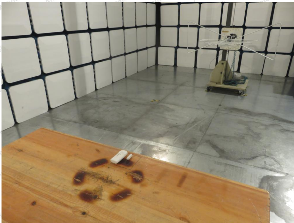
Photo of Radiation Emission Test
