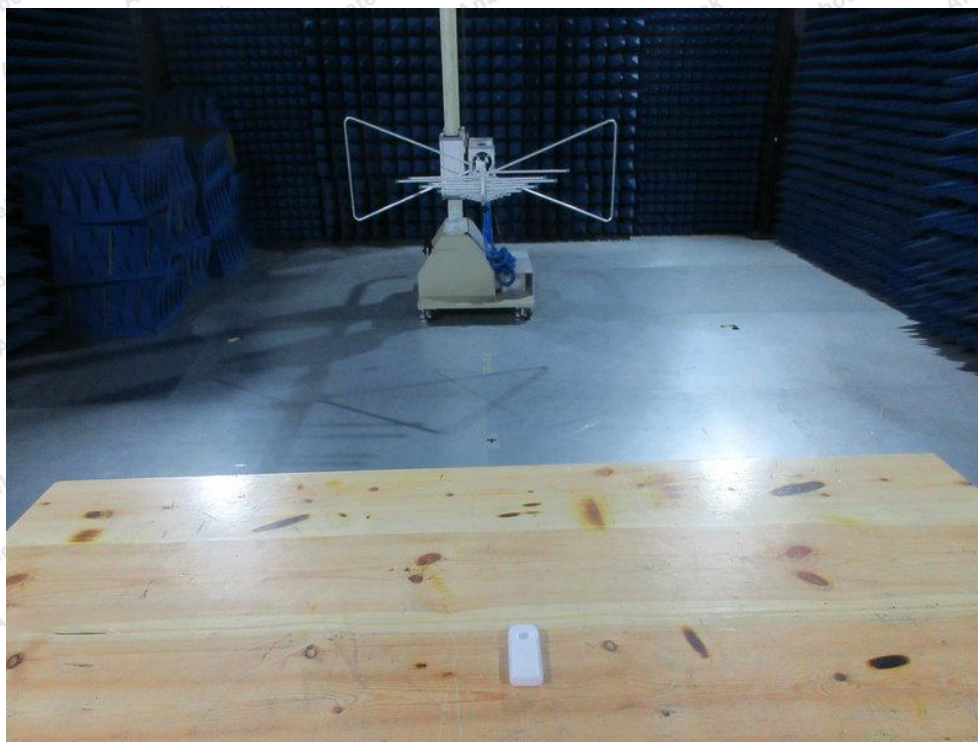
Photo of Radiation Emission Test
