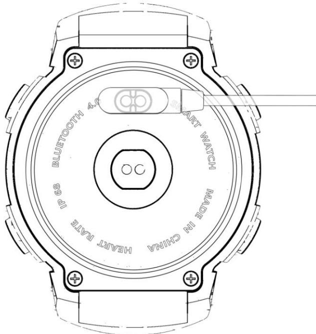
**Please note that the two contacts of the charging cable can not touch the conductive object at the same time, otherwise it will cause short circuit combustion.**
