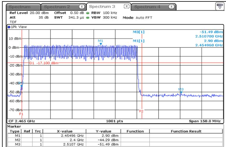
**- Result of 2 400.0 MHz - 2 483.5 MHz****- 8DPSK (Without hopping)**
