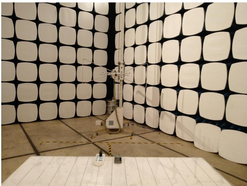
RADIATED EMISSION ABOVE 1G TEST SETUP
