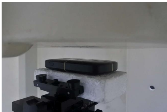
Front, Test Separation 19mm
