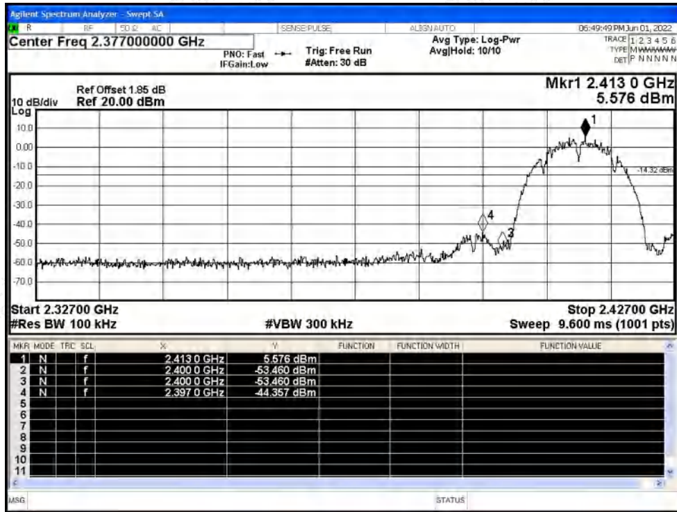
Band Edge NVNT b 2412MHz Ant1 Emission
