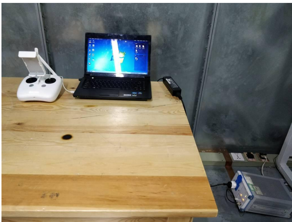
Fig. 2 AC Conducted Emission of charge from PC mode
