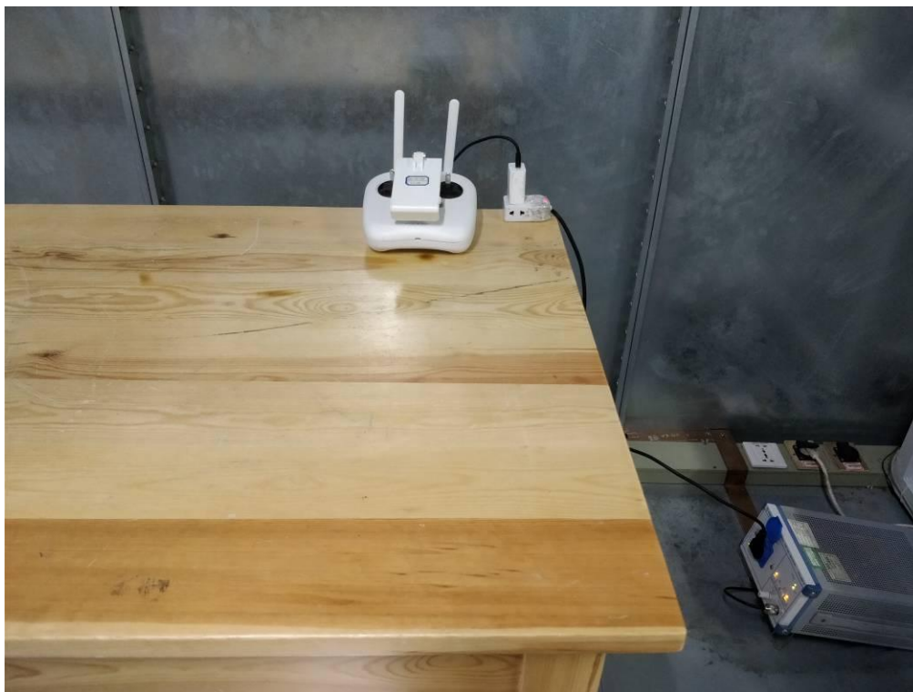
Fig. 1 AC Conducted Emission of charge from power adapter mode
