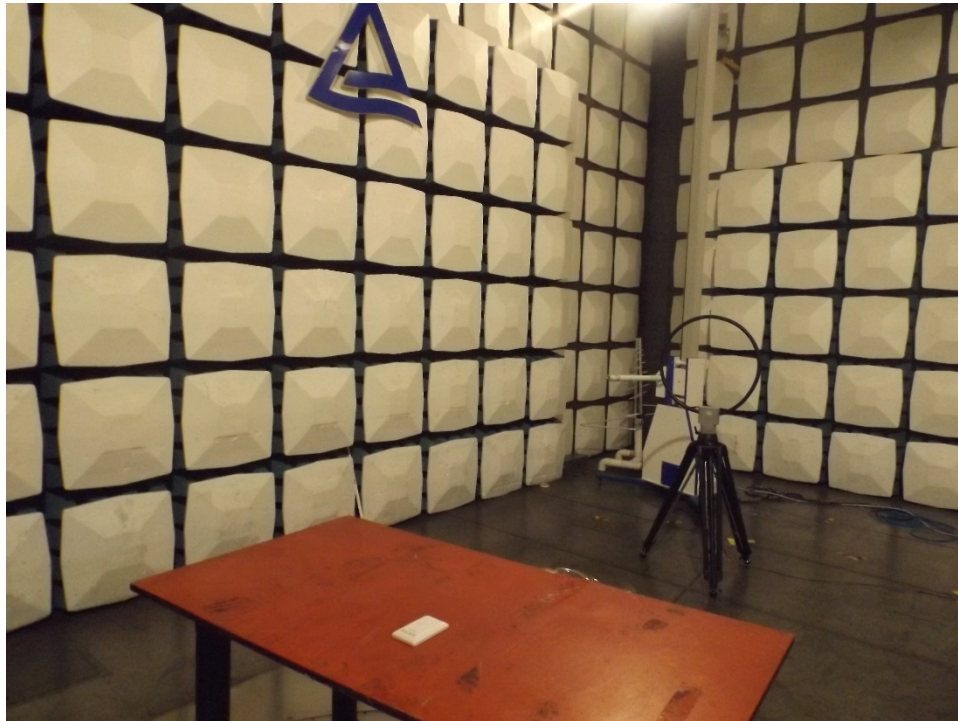
Photograph 1: Set-up for Radiated Spurious Emission, 9kHz - 30MHz
