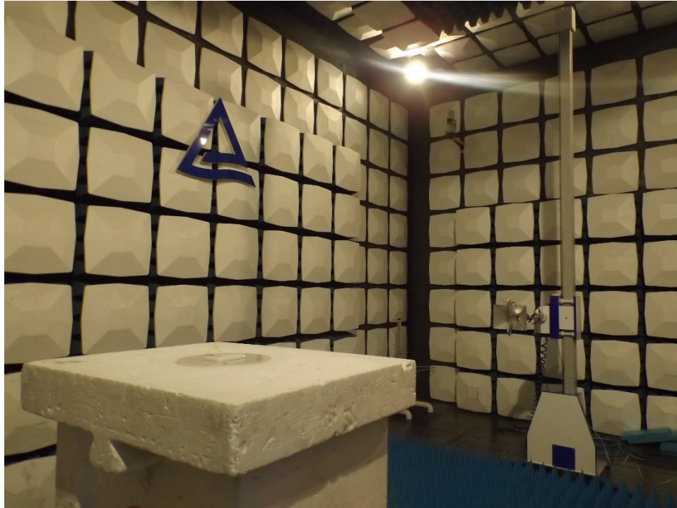
Photograph 3: Set-up for Radiated Spurious Emission, 1GHz - 5GHz
