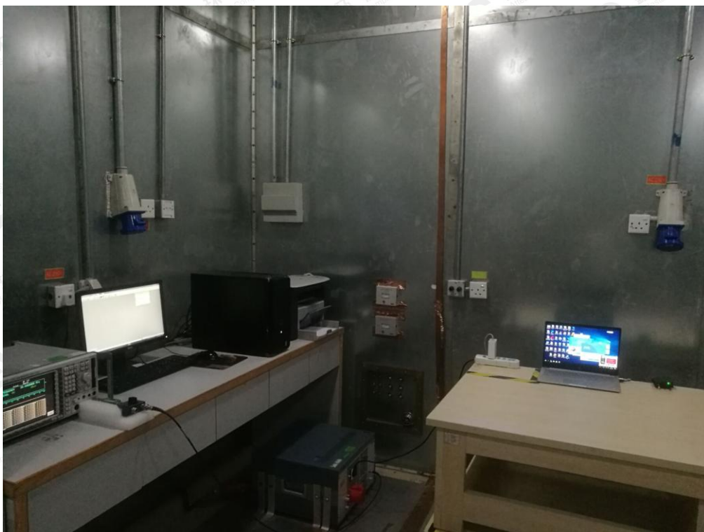
FCC RADIATED EMISSION TEST SETUP BELOW 1GHZ
