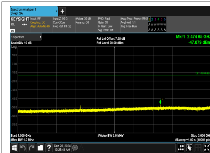
Band26(824-849)-15MHz-16QAM-26865-1RB#0-1000~3000-PASS
