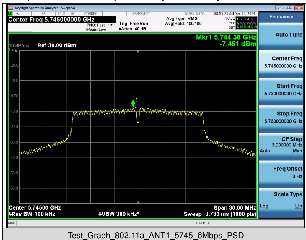
Test Graphs of Conducted Output Power Spectral Density for band 5.725-5.85 GHz
