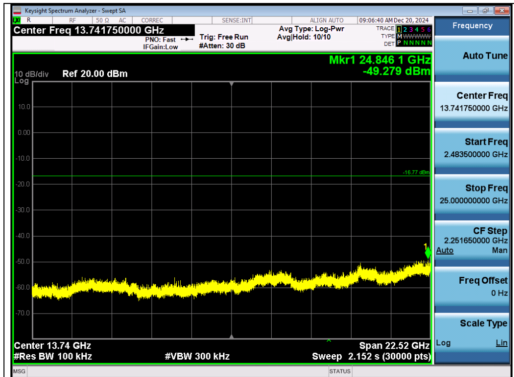
Test_Graph_EDR_ANT1_2441_2Mbps_Higher Band Emissions
