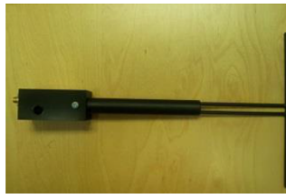
Figure 1 – MVG COMOSAR Validation Dipole
