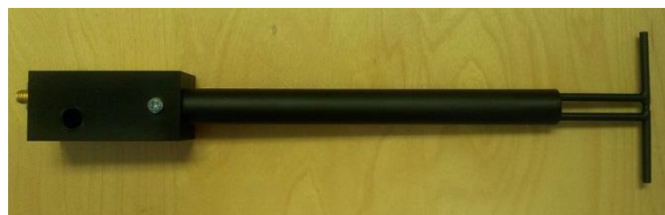
Figure 1 – MVG COMOSAR Validation Dipole
