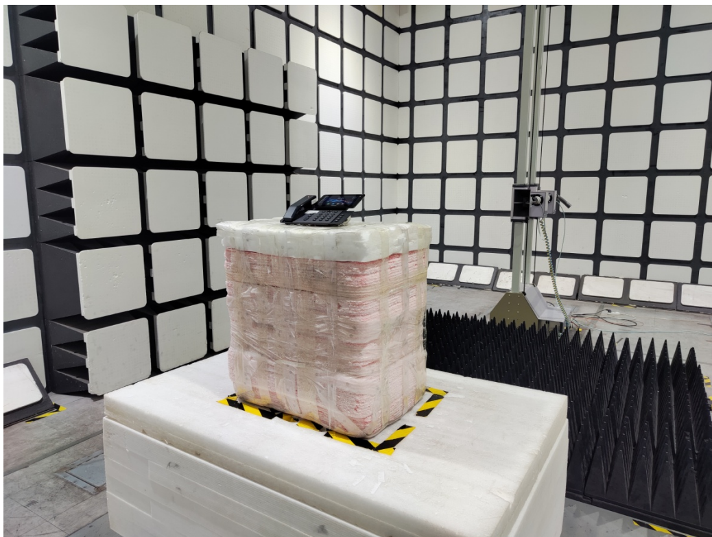
Radiated Emissions View (1-18 GHz)
