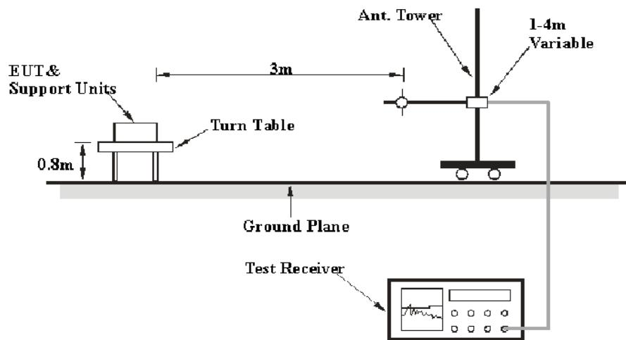
The radiated emission tests were performed in the 3 meters test site, using the setup accordance with the ANSI C63.10-2013 & RSS-Gen. The specification used was the FCC 15.209, and FCC 15.247 & RSS-Gen limits.
