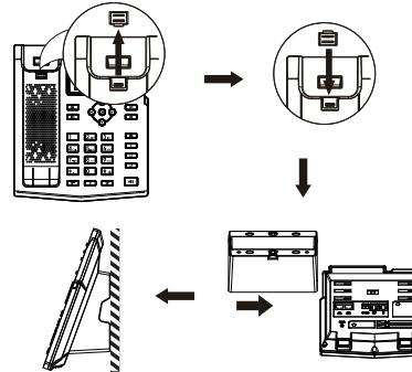
Note: The installation height of the wall-mounted bracket is less than 2 meters from the ground.
