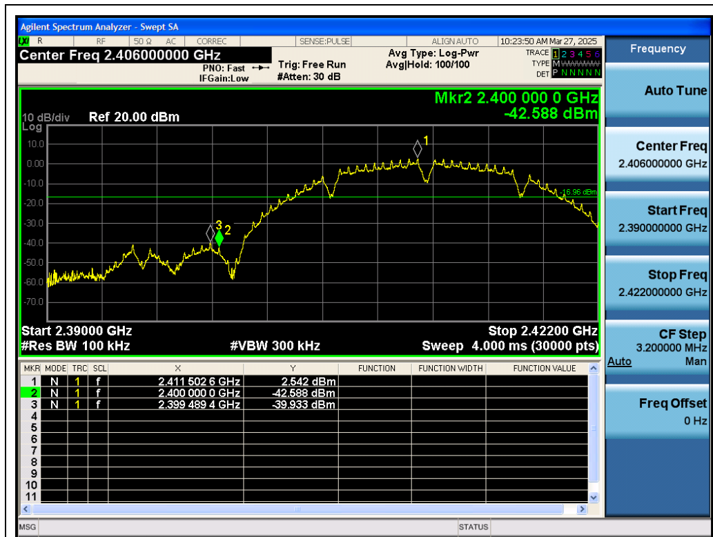
Test_Graph_802.11b_ANT2_2412_1Mbps_Lower Band Edge Emissions
