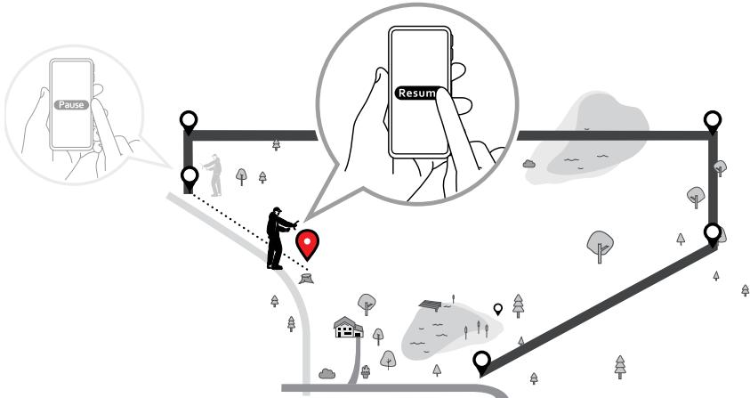
For large fences of 5 acres or more, use the Pause function to manually control the number of fence posts, so you don't run out. This will also reduce the fence file size and help the fence load faster.
