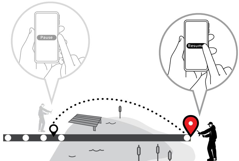
Hit an obstacle you can't walk through, like a pond or thick brush? Using the app press Pause to manually drop your next fence post, go around the obstacle and then press Resume. SpotOn will snap a fence line between fence posts.
