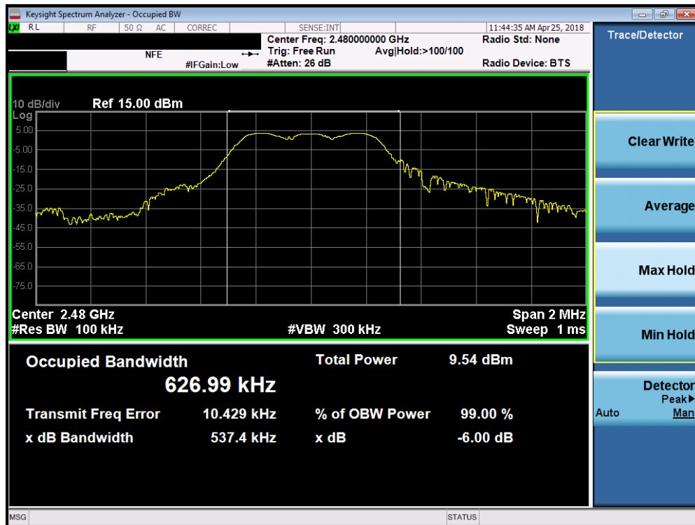
Plot 7-3. 6dB Bandwidth Plot (Bluetooth (LE), 250kbps – Ch. 39)
