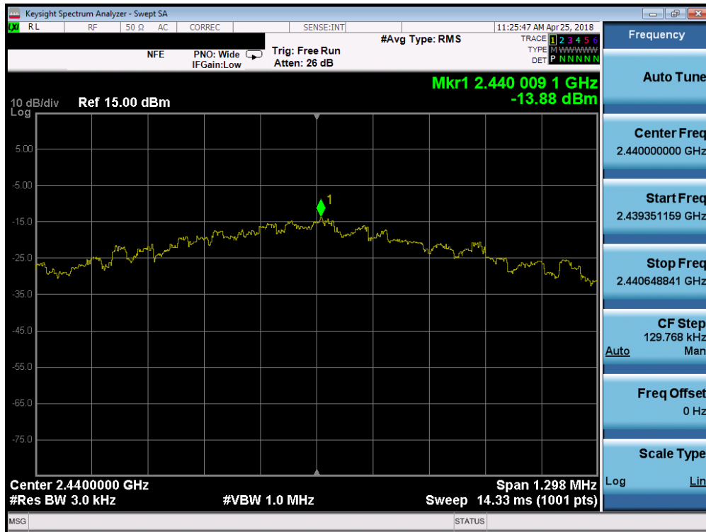
Plot 7-26. Power Spectral Density Plot (Bluetooth (LE), 2Mbps – Ch. 19)
