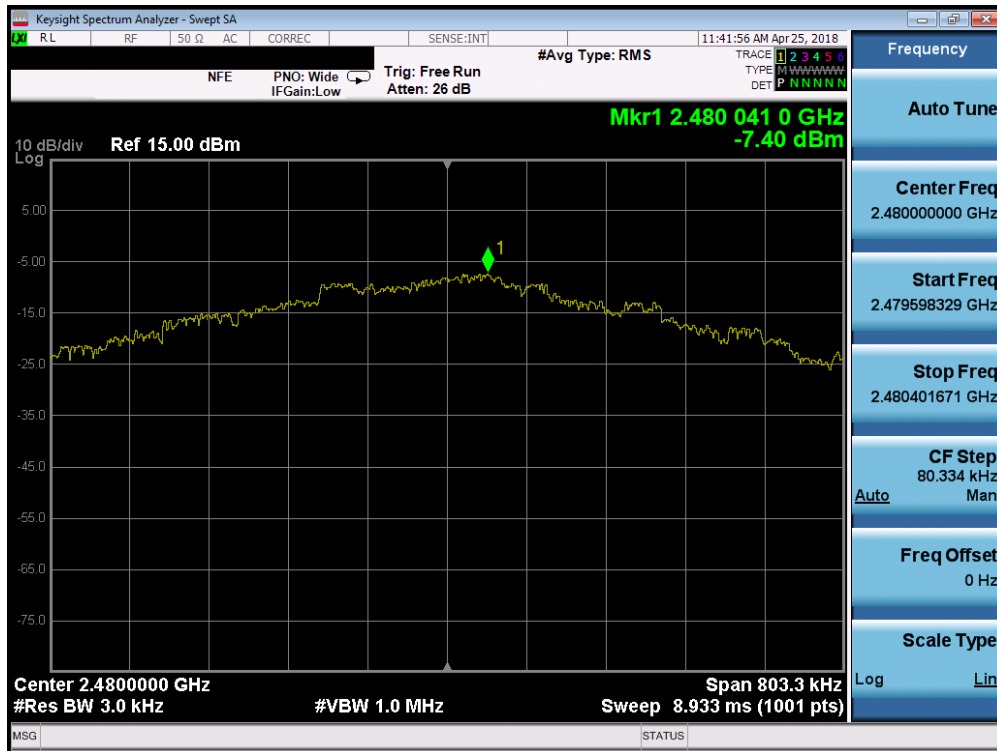
Plot 7-24. Power Spectral Density Plot (Bluetooth (LE), 1Mbps – Ch. 39)
