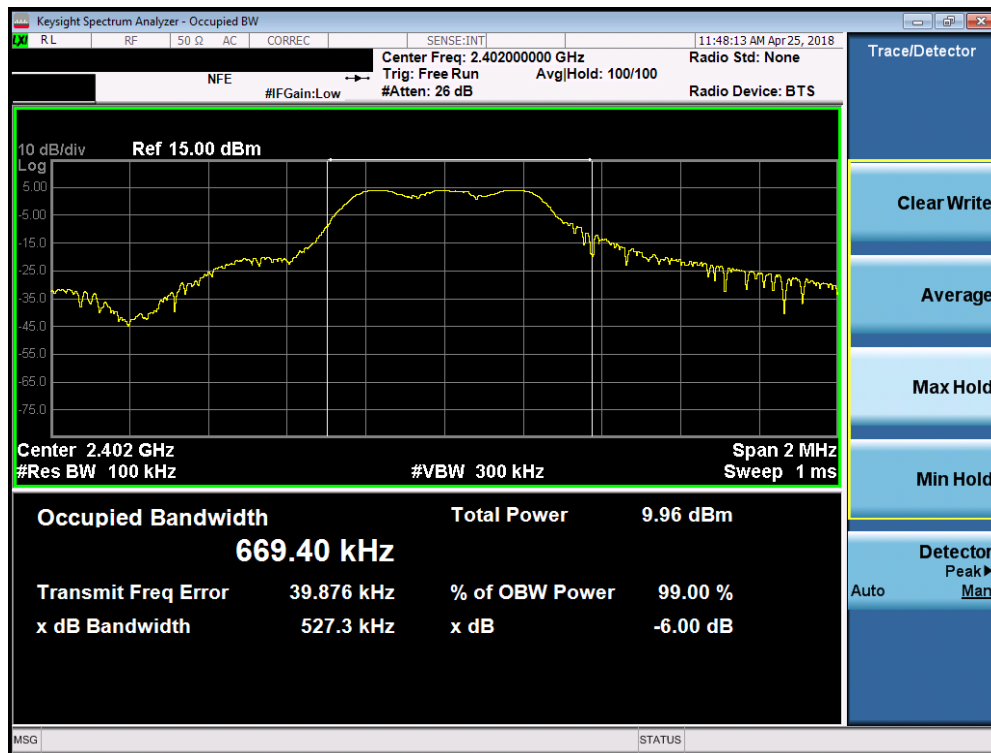
Plot 7-1. 6dB Bandwidth Plot (Bluetooth (LE), 250kbps – Ch. 0)
