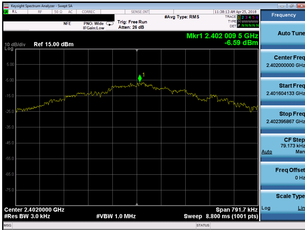
Plot 7-22. Power Spectral Density Plot (Bluetooth (LE), 1Mbps – Ch. 0)
