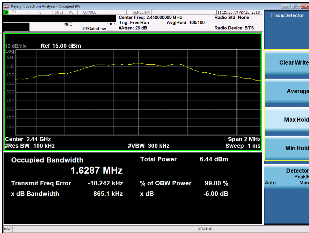
Plot 7-8. 6dB Bandwidth Plot (Bluetooth (LE), 2Mbps – Ch. 19)
