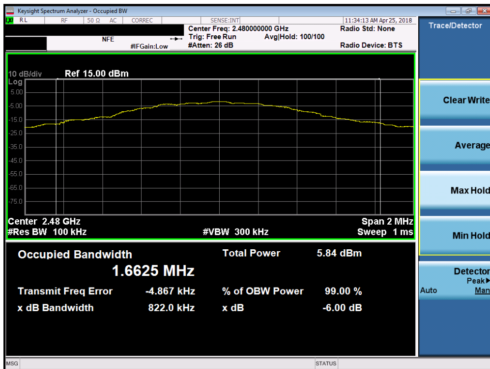
Plot 7-9. 6dB Bandwidth Plot (Bluetooth (LE), 2Mbps – Ch. 39)
