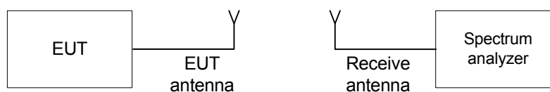
Figure 7.2.1 Carrier frequency separation test setup
