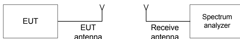
Figure 7.2.1 Carrier frequency separation test setup
