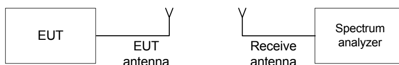
Figure 7.3.1 Hopping frequencies test setup
