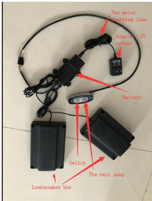
The system consists of left and right channels of high quality speakers, a Bluetooth power amplifier board, a charger, charging lines and switches. (Horn and Bluetooth power amplifier board are hidden in office chairs)
