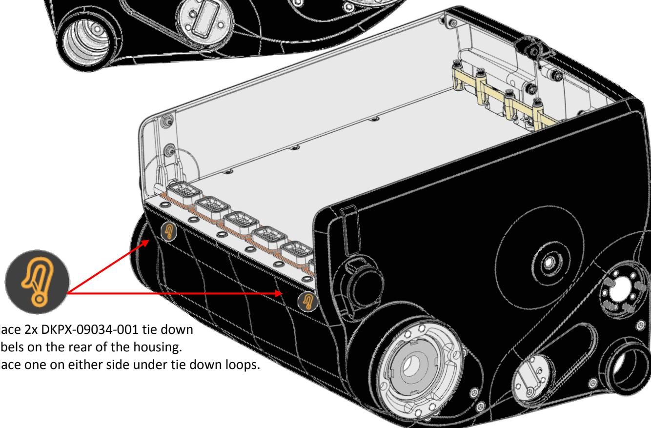
Place 2x DKPX-09034-001 tie down labels on the rear of the housing.
