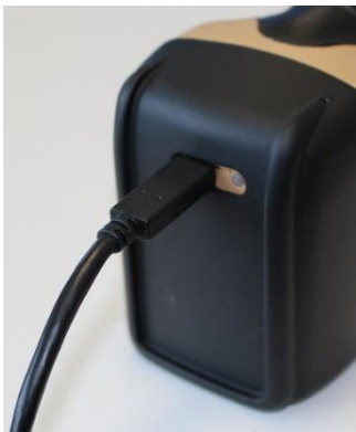
Figure 8: Location of the USB-C Receptacle
