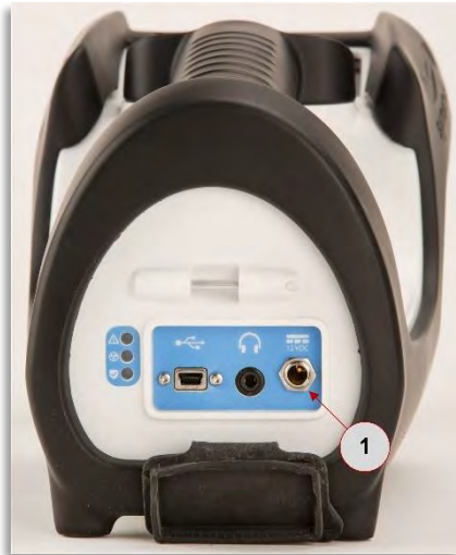
Figure 25: Location of the Power Receptacle
