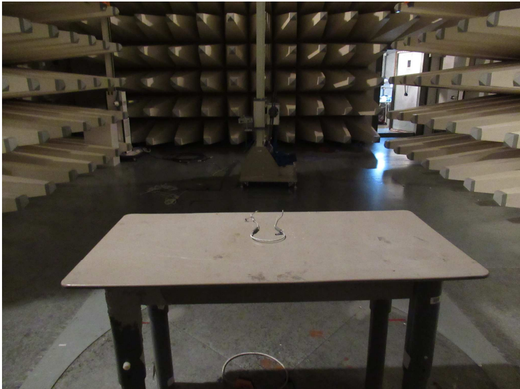
Set-up for Radiated Emission
