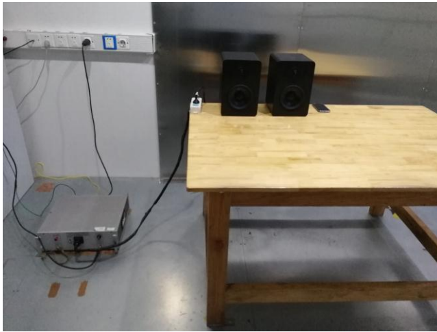
Conducted Emissions Test Setup Front View
