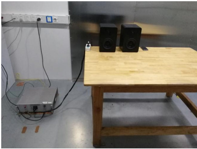
Conducted Emissions Test Setup Front View
