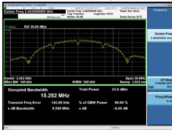
802.11b, Carrier frequency (MHz): 2462
