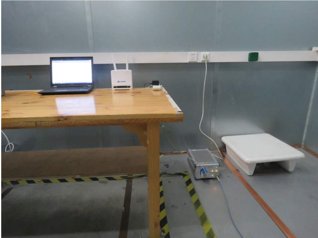
Conducted Emission Test Setup
