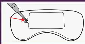
Remove battery cover from the underside of the remote with a phillips head screwdriver (not included), as shown.
