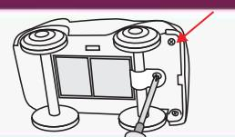
Remove battery cover from the underside of the car with a phillips head screwdriver (not included), as shown.
