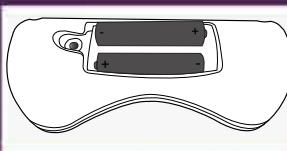
Insert (2) AAA batteries (not included) as shown in battery compartment, and replace battery cover.
