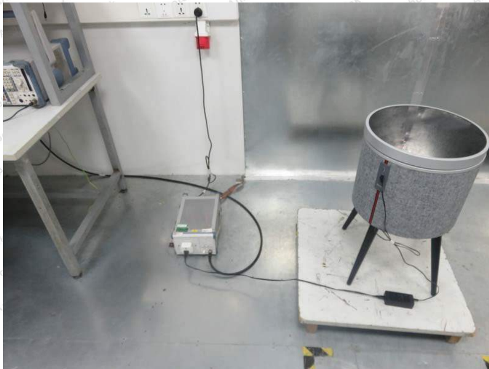
Photo of Conducted Emission Measurement
