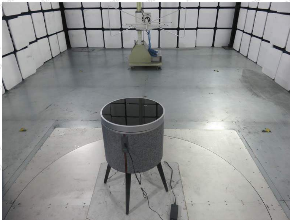
Photo of Radiation Emission Test
