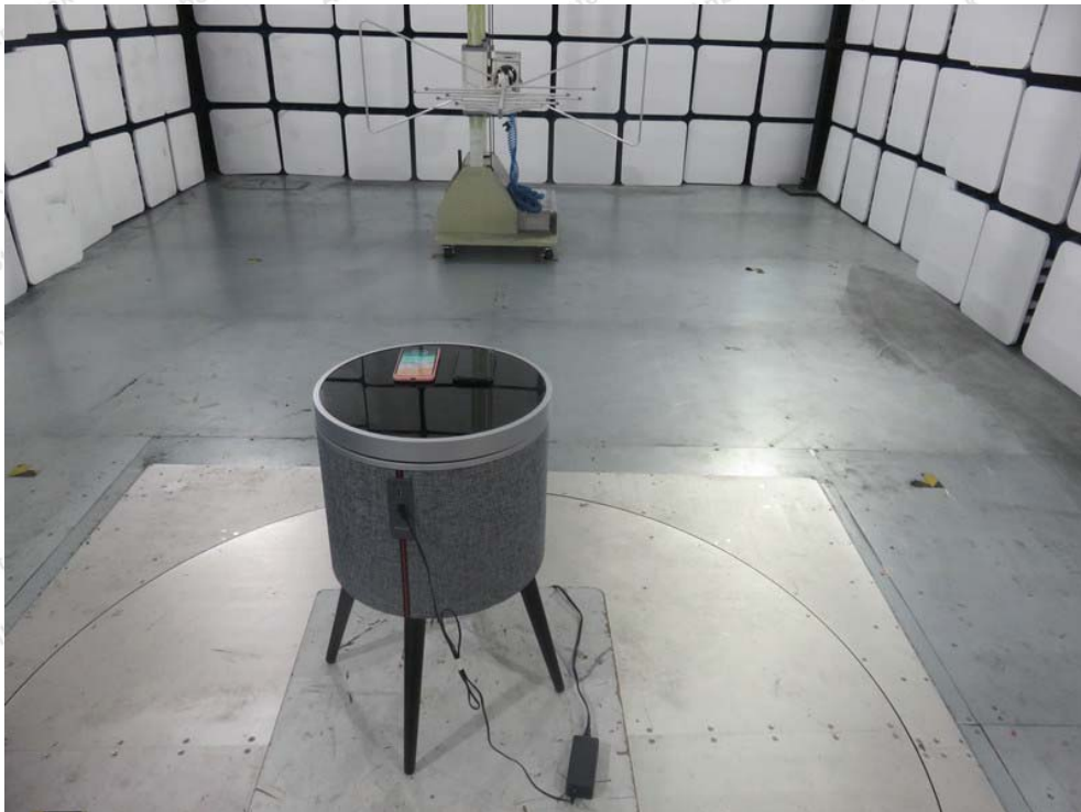
Photo of Radiation Emission Test
