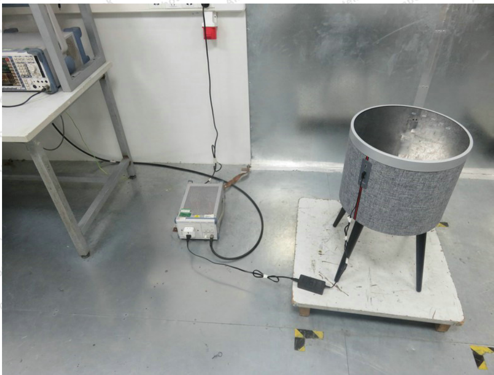
Photo of Conducted Emission Measurement
