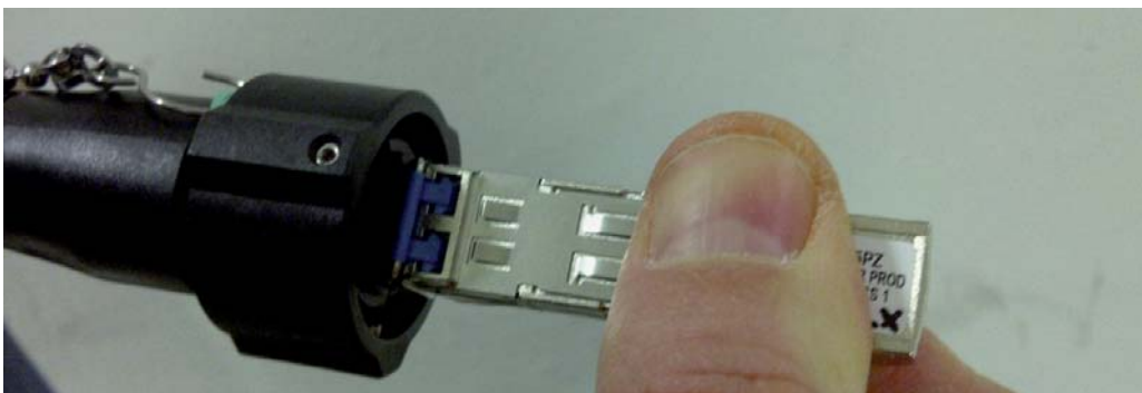
Fig.73 - Amphenol SFP/LC connector check
