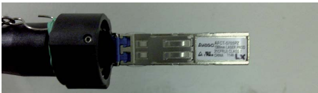
Fig.72 - Amphenol SFP/LC connector locked
