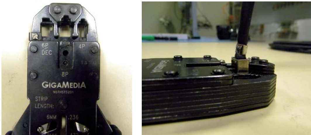
Fig.45 - Standard RJ45 crimper (without comb) used for RJ45 shielded outdoor connector
