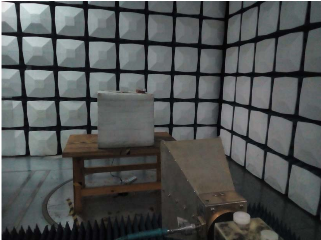
Radiated Emission Above 1GHz View
