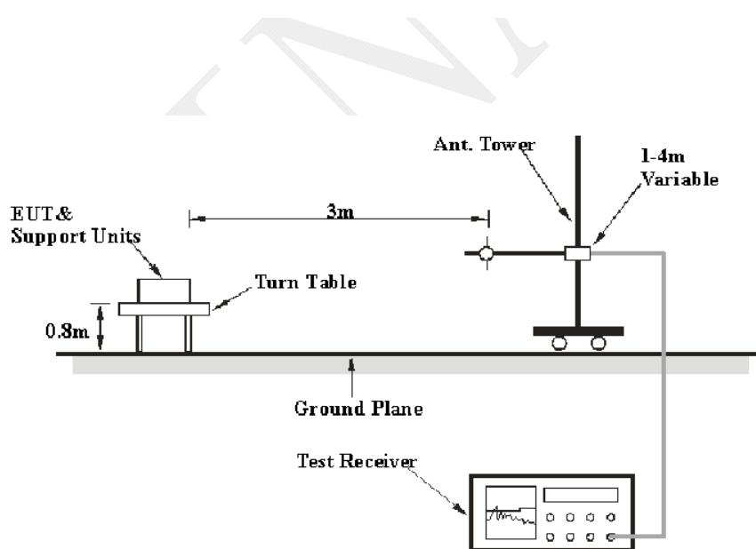
The radiated emission tests were performed in the 3-meter chamber test site, using the setup accordance with the ANSI C63.10-2013. The specification used was the FCC Part Subpart C limits.
