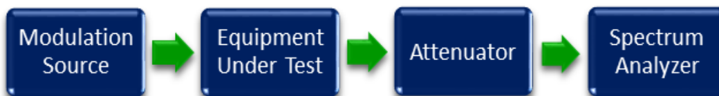
Figure 3: Occupied Bandwidth Test Setup
