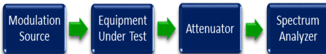
Figure 2: Modulation Characteristics Bandwidth Test Setup
