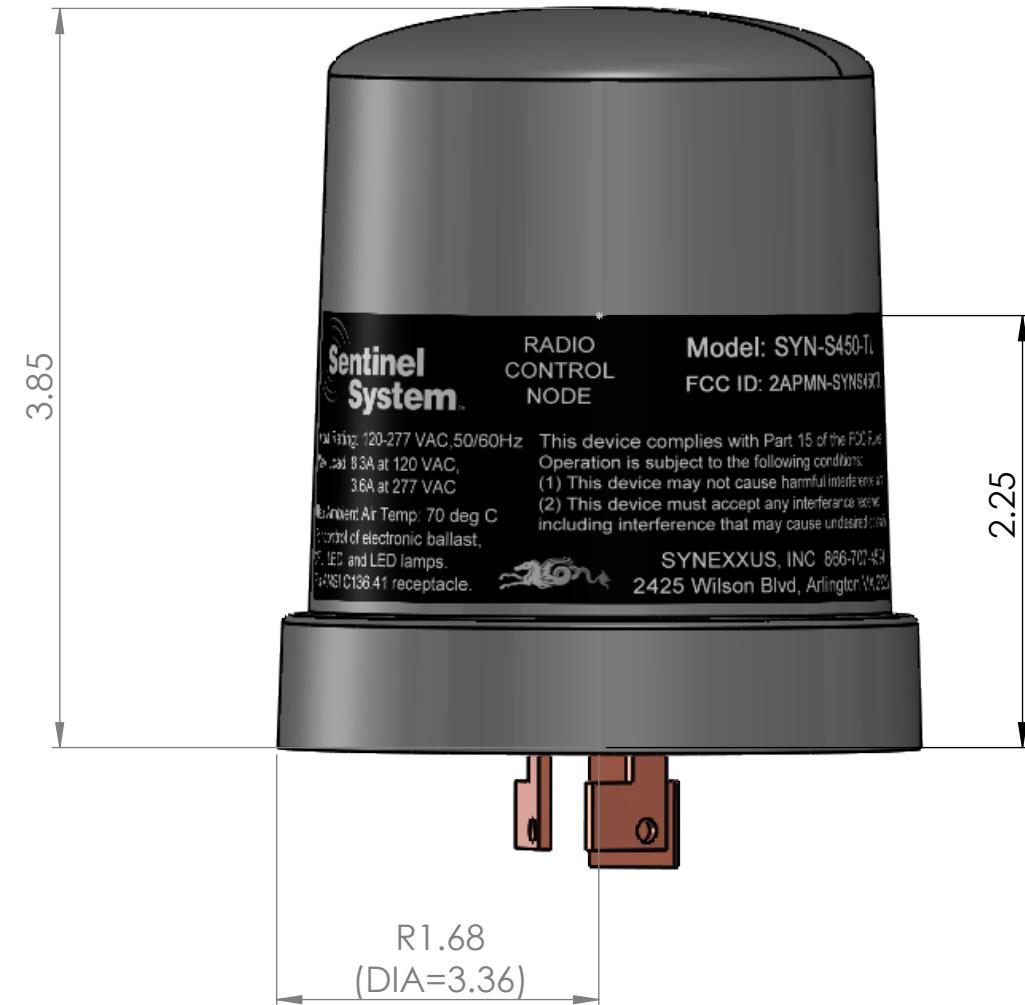
Label vertical position dimension is shown. The label is attached parallel to the plug interface plane. The label may be rotated at any orientation with respect to the centerline axis.
