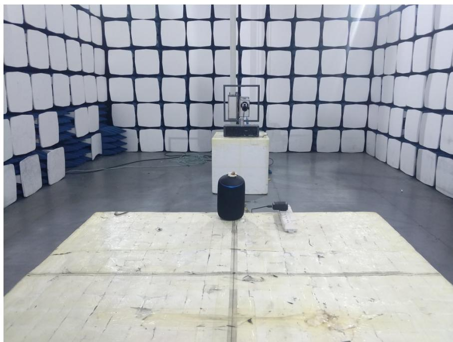
**Radiation Emission Test Setup (30MHz to 1GHz)**
