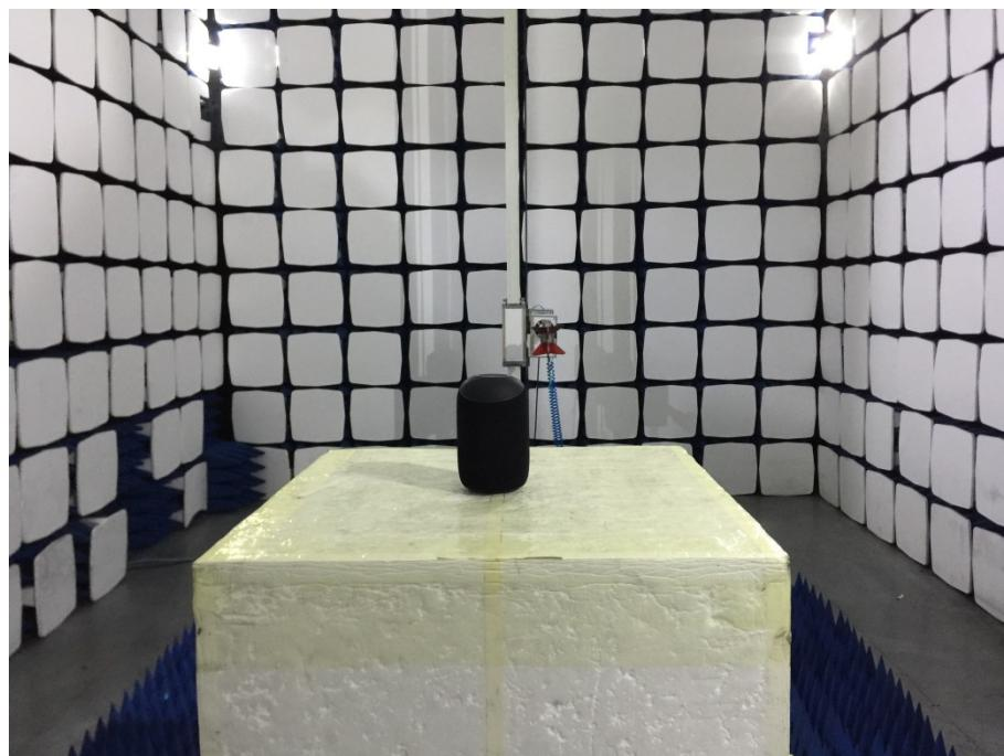
**Radiation Emission Test Setup (Above 18GHz)**
