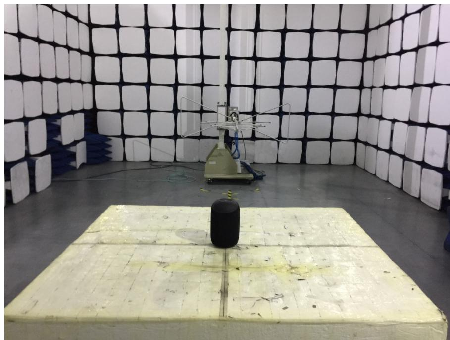
**Radiation Emission Test Setup (1GHz to 18GHz)**
