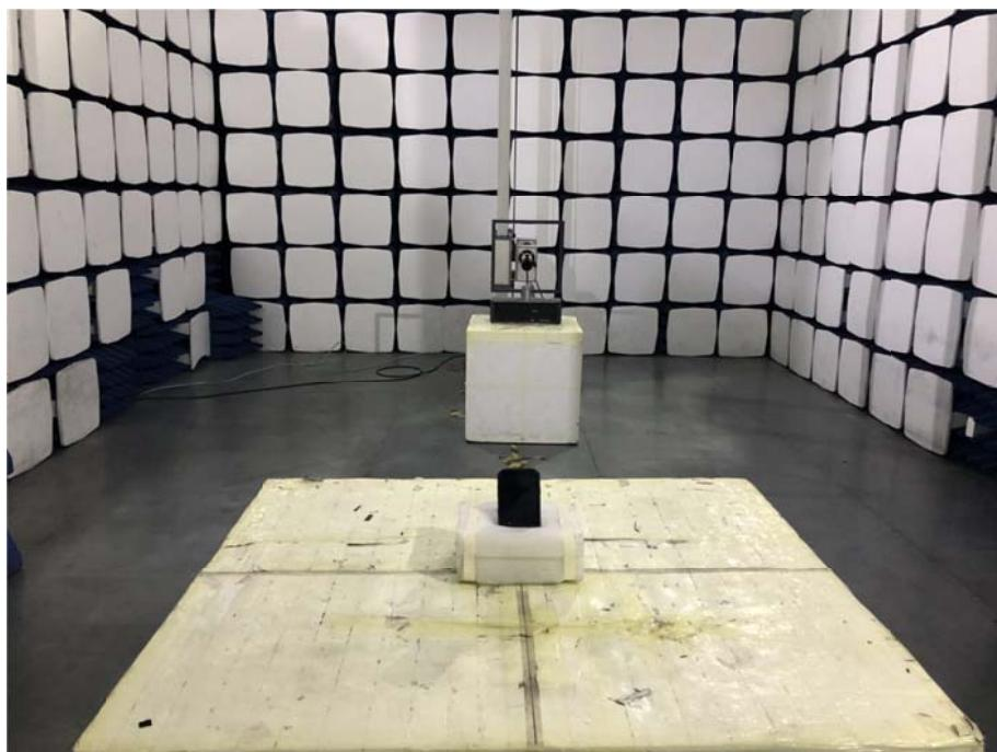
**Radiation Emission Test Setup (30MHz to 1GHz)**
