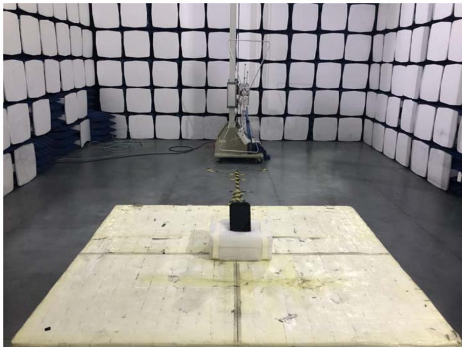
**Radiation Emission Test Setup (1GHz to 18GHz)**
