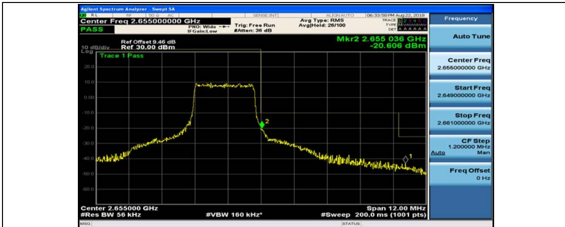
(Channel Bandwidth: 5 MHz)_HCH_QPSK_25RB#0
