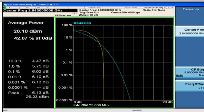
(Channel Bandwidth:20 MHz)_HCH_QPSK_50RB#0
