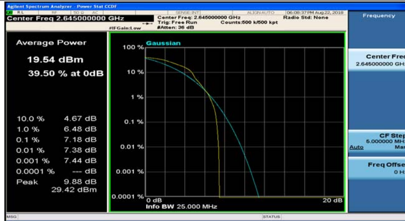
(Channel Bandwidth:20 MHz)_HCH_16QAM_1RB#49
